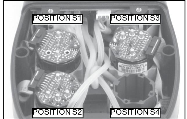
The upgrading of the number of sensors can be easily done by the user by performing the following directions:
