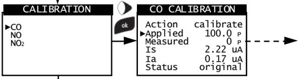
The installed sensors are shown, and can be chosen for recalibration. In the calibration screenshot, information about the calibration in use and sensor output are displayed.
