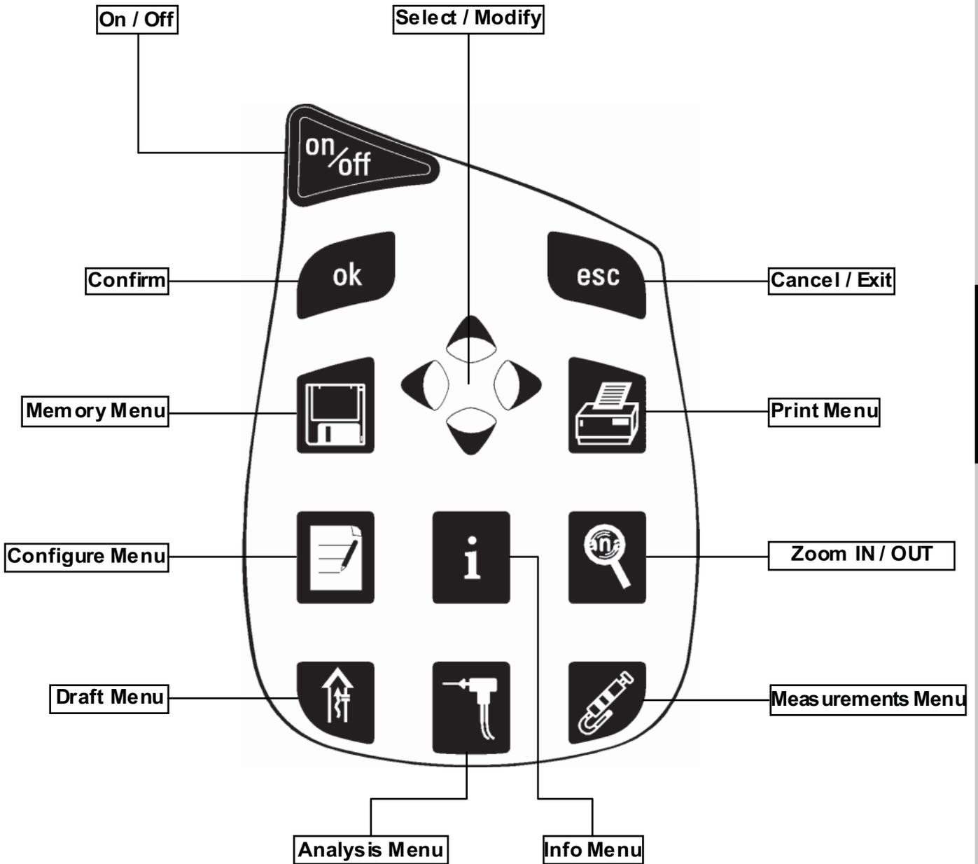
**WARNING:** to turn-on / off the instrument it is necessary to press and hold the On/Off button for at least 2 seconds.
